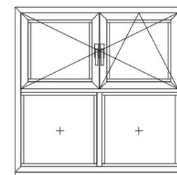
A pivoting casement, a pivoting / tilt casement and two fixed casements
