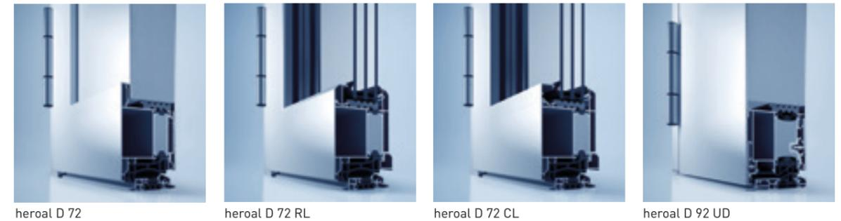
Whether with standard outer contours (**heroyal D 72**), rounded-off Roundline contours (**heroyal D 72 RL**) or bevelled Classicline contours (**heroyal D 72 CL**), heroyal door systems with a design depth of 72 mm are ideally suited for both new buildings and renovation. The entrance door system **heroyal D 92 UD** offers high heat insulation values up to suitability for passive houses.
